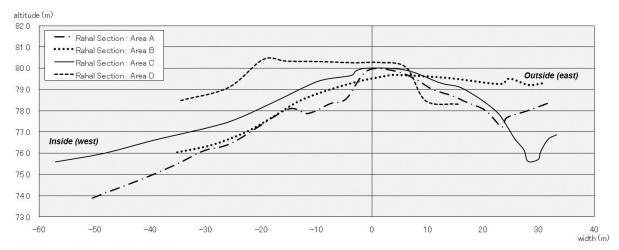
Figure 9: Cross sections of east side embankment of Rahal
