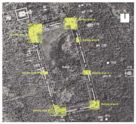
Figure 8: Surveyed area on the surrounding embankment of Rahal; topographical survey was conducted in 7 areas A to G, and a west-east cross section survey was conducted in area A to D.
