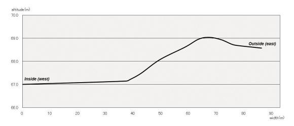
Figure 10: Cross section of east side embankment of north reservoir KK109
