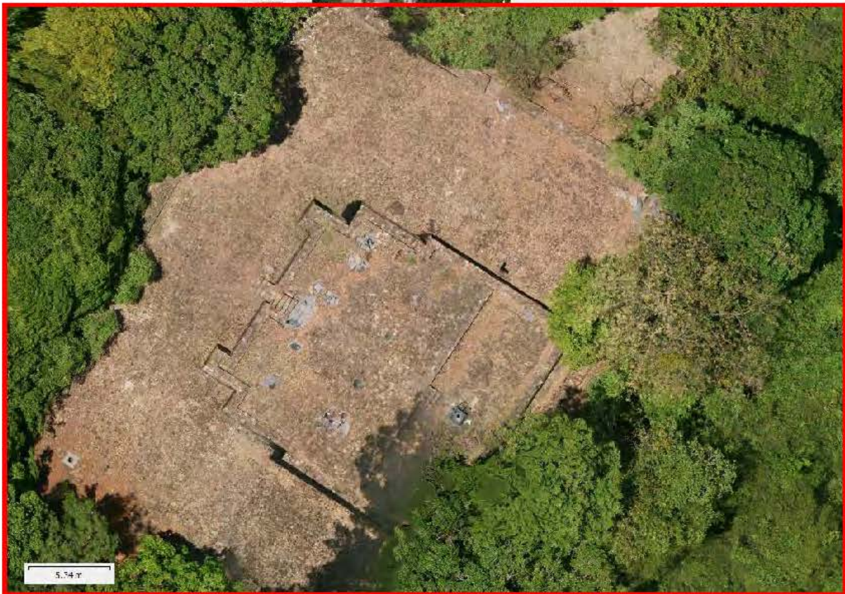
Figure 5.18: Monument No. 2 (largest brick structure) at Khao Kha, generated using SfM Technique
