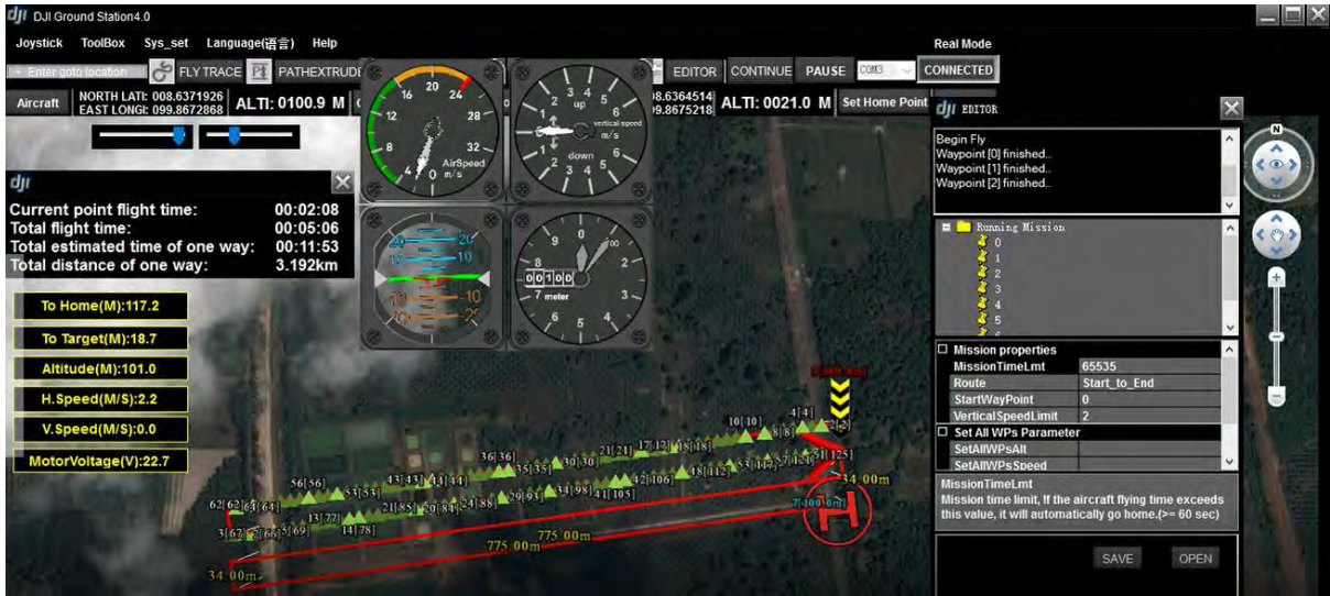
Figure 5.6: PC ground station control UAV autopilot for taking pictures along each flight plan
