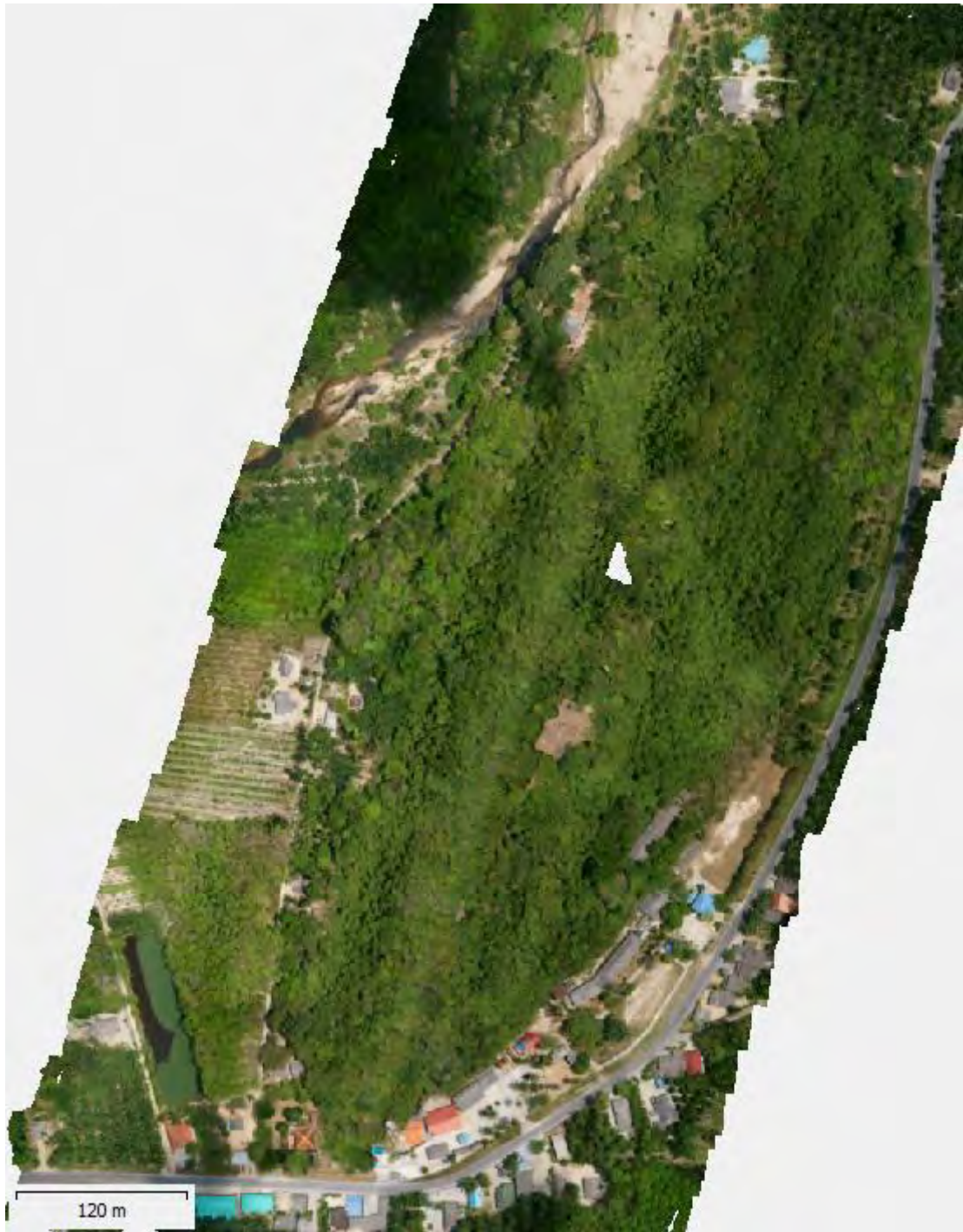
Figure 5.15: Image of Khao Kha generated using drone and SfM Technique
