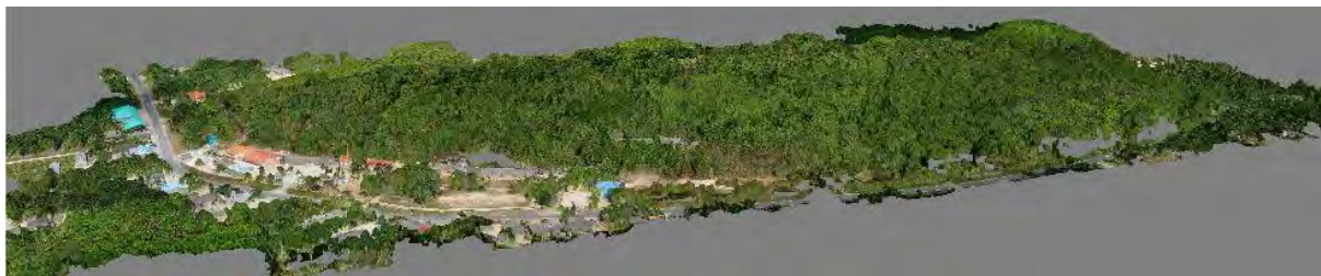
Figure 5.8: High resolution 3D image map from SfM technique
