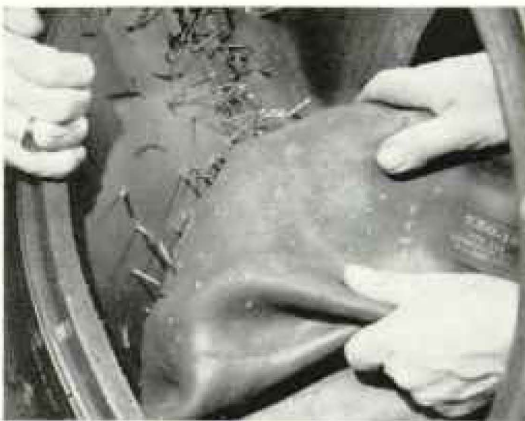
3. Seiberling Sealed-Air Tube being removed from tire for inspection after being pierced with more nails than you'll ever pick up. Each raised "rubber rivet" marks a spot where tube has permanently repaired itself! It's safe for many more thousands of miles of driving.
